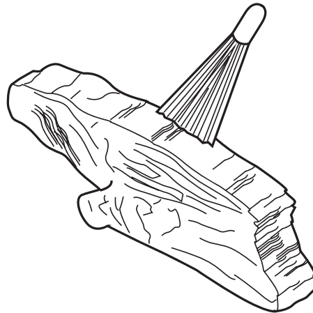
Figure 36 - Removing Soot with a Soft Bristle Brush
